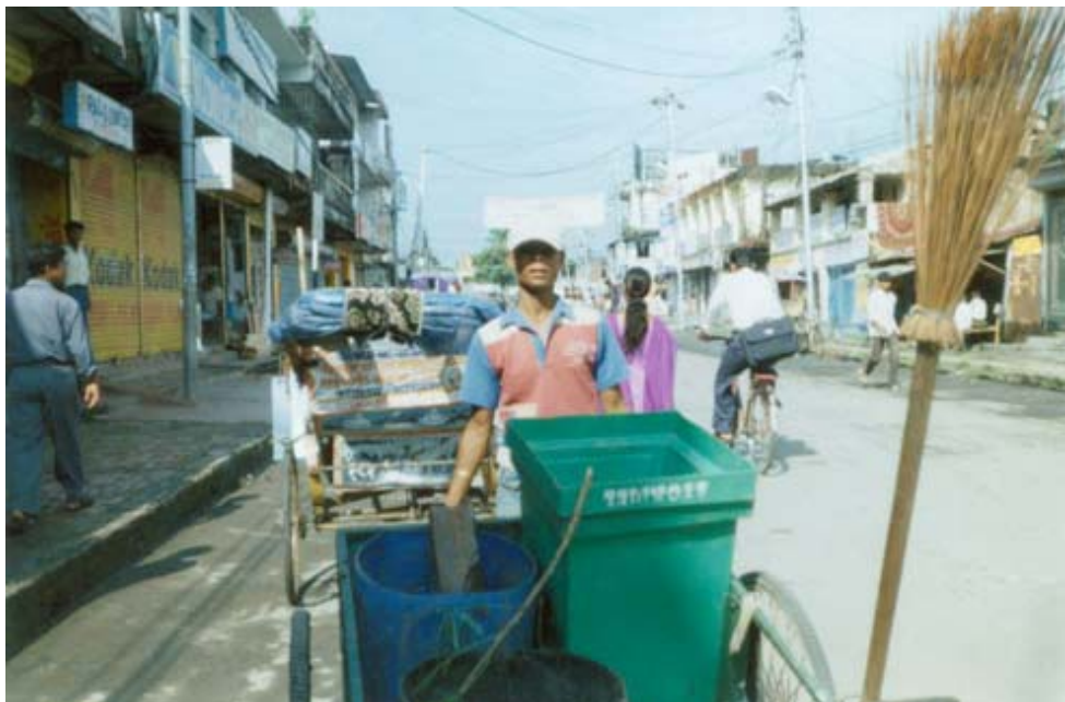
A Hand Cart Used for Waste Collection
