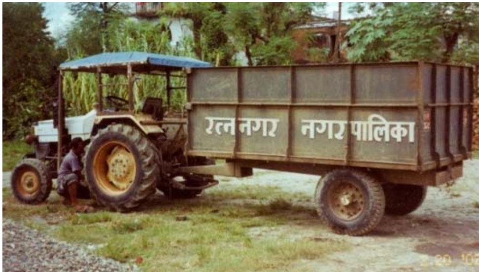
**Tractor with Modified Trailer to Accommodate Large Amount of Waste**
