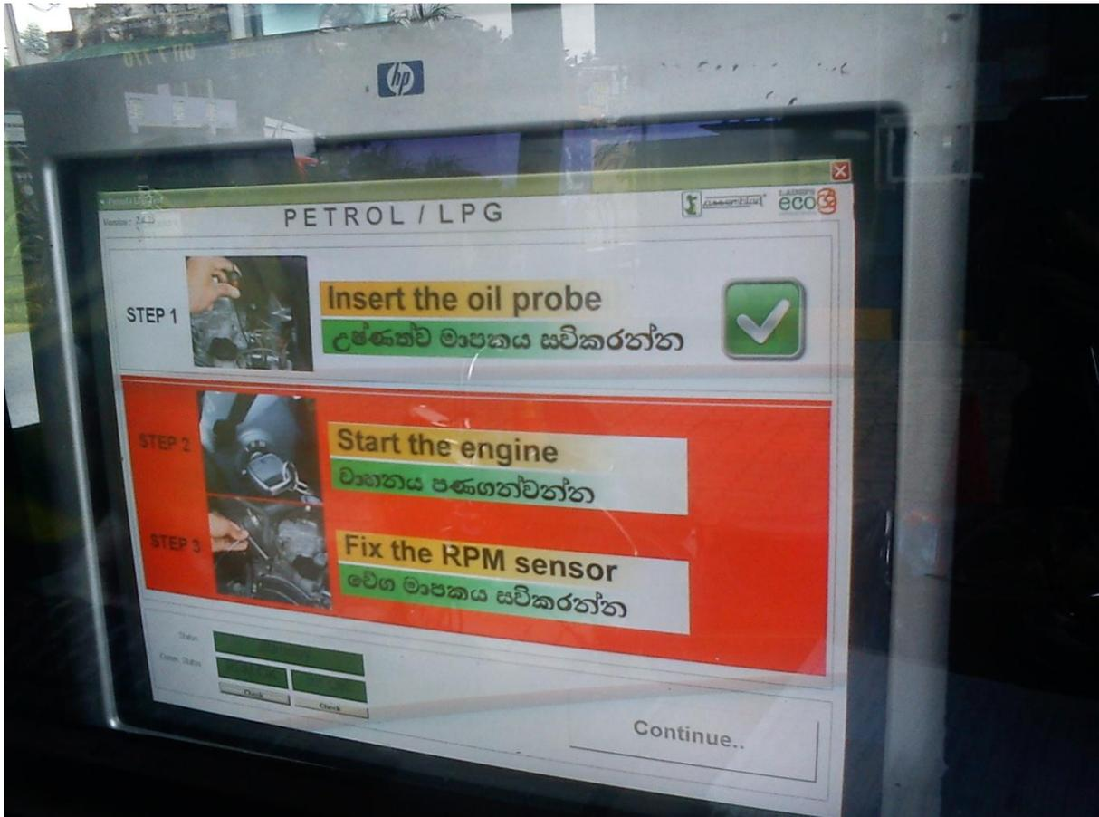
PHOTO 4 : The automated Software providing guidance to the technicians
