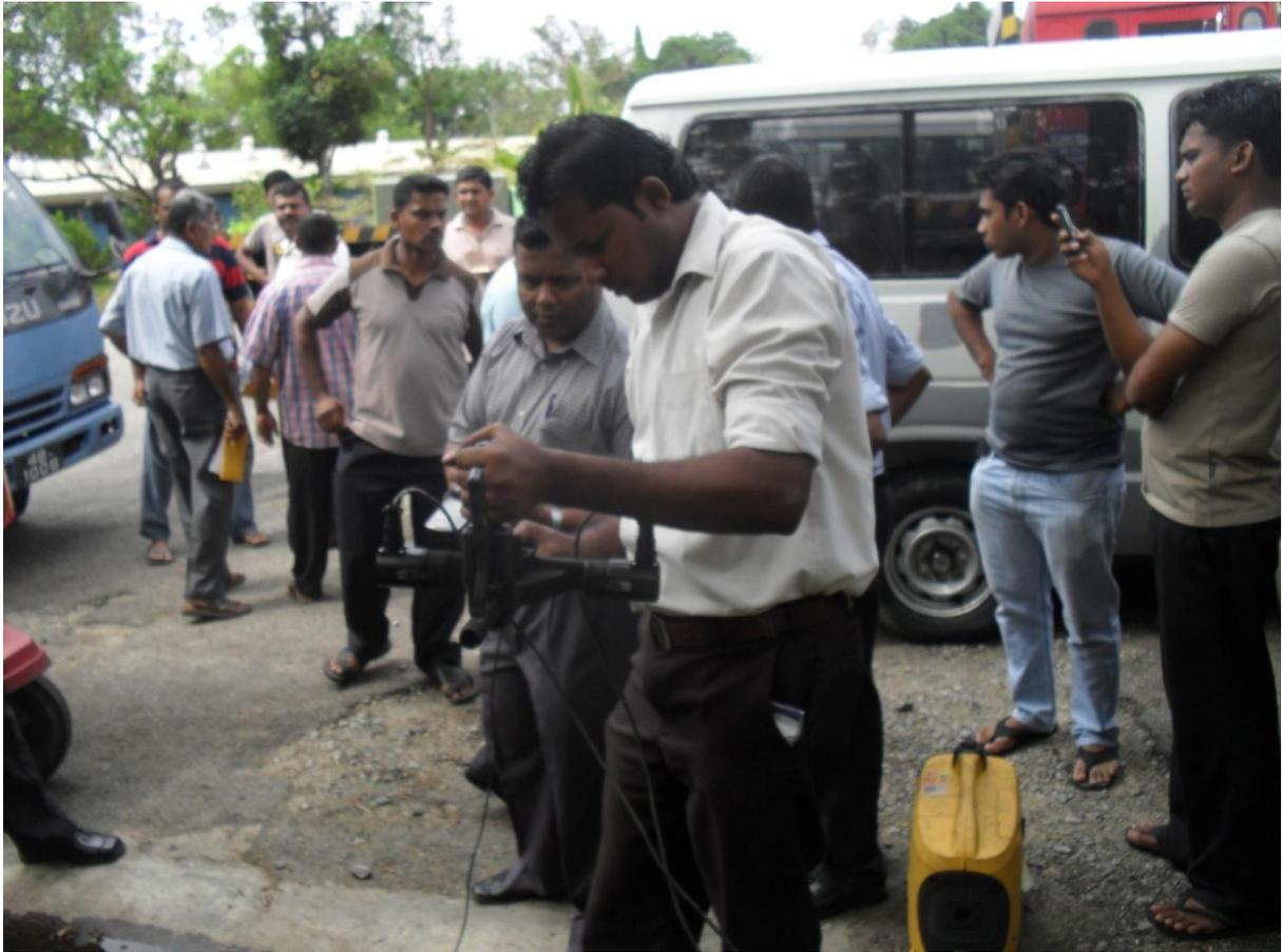
PHOTOS 9 Calibrating the Smoke meter during Smoky Vehicle Emission Testing Program
