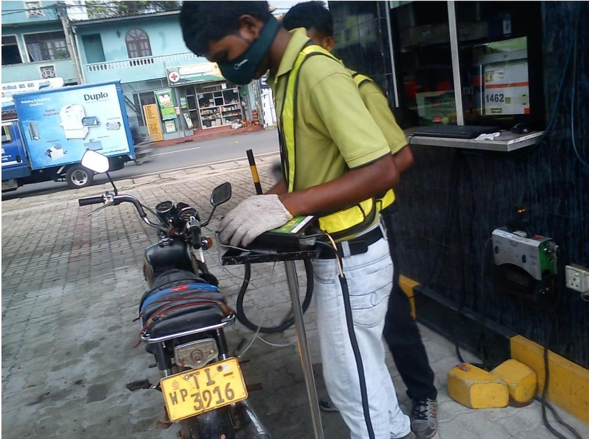
PHOTO 5 : Emission testing of a two-wheeler vehicle
